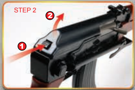
STEP 2 1.Push Receiver top catch and hold. 2.Remove the Receiver top cover.
