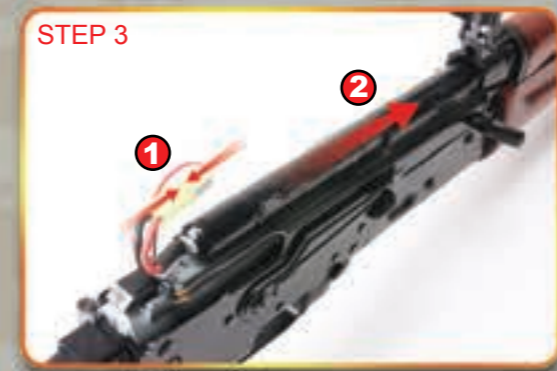
STEP 3 1.Connect the battery leads. 2.Insert the battery .
